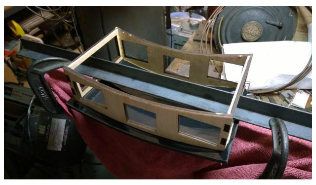
Construct a cupola roof and attach the cupola to the roof. Depending on how you construct your roof, this is the last time to have access to the interior of the cupola.
