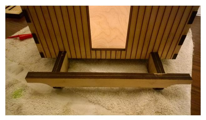
Glue and clamp the end sills to the tabs on the end of the frame beams. The untabbed end sills should be glued to the ends covering the tabs.
