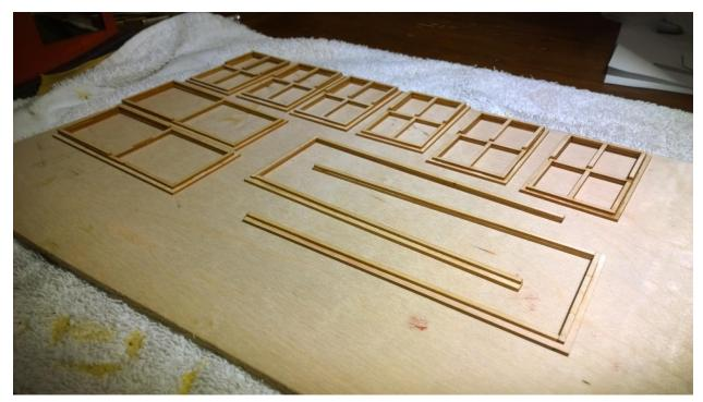
Glue the door frames together. Once dry, it is a good time to paint or stain the door frames.
