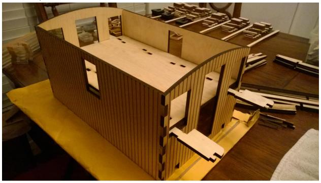
Glue the main walls together. To ensure a square body, suspend the floor in the body supporting it with the frame beams resting through the end windows
